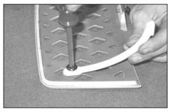
Figure 8.21 Install warming shelf bracket loosely to each warming shelf using the bolt provided.
